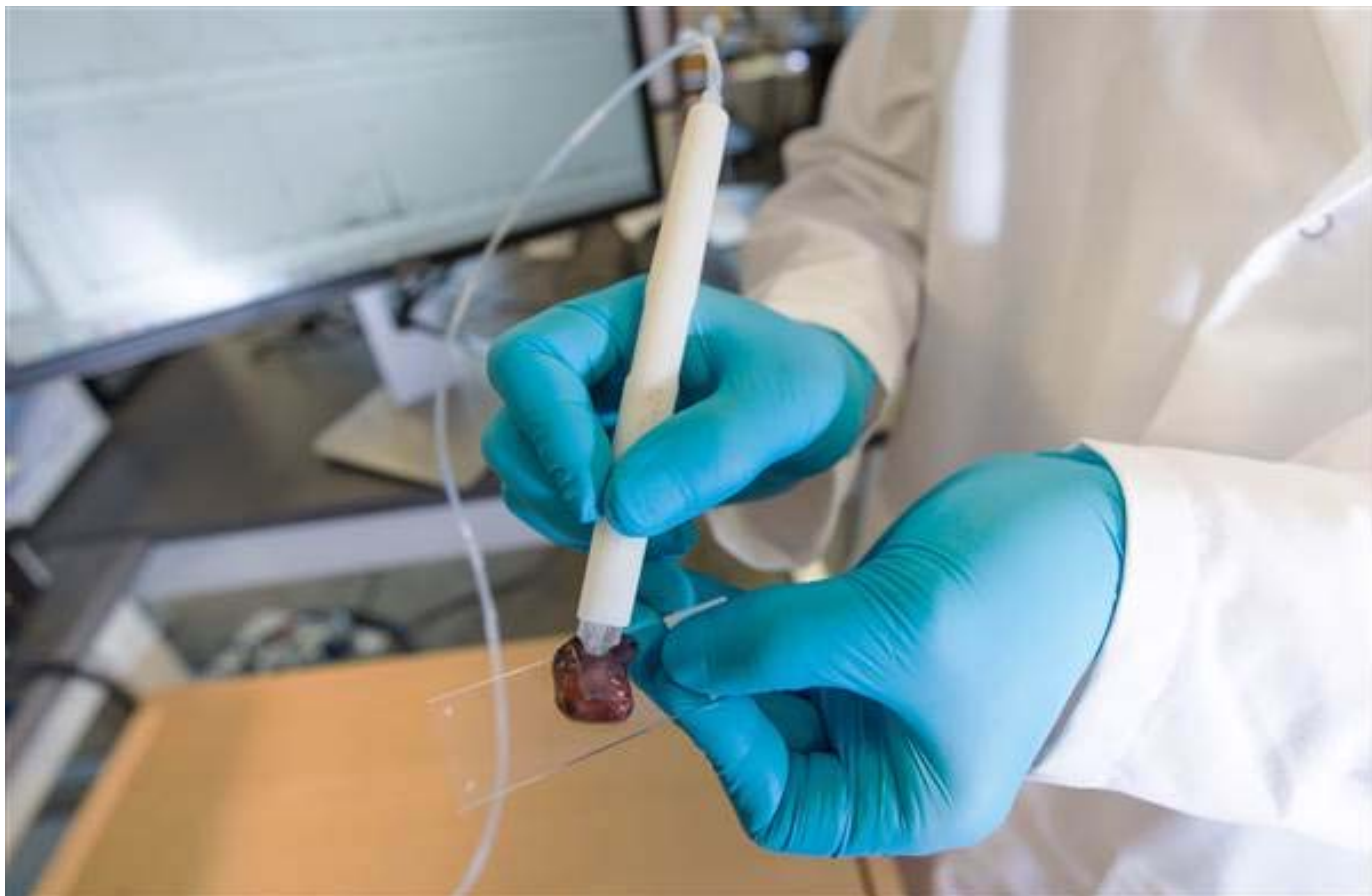
The MasSpec Pen is a handheld probe that can non-destructively analyze human tissue samples to identify cancer. Vivian Abaigu/University of Texas at Austin
